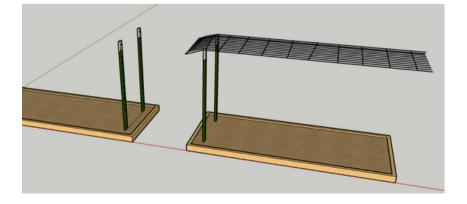
Orient the cattle panel horizontally so that it is parallel to the ground. Begin carrying the panel over to the T-posts. Position the panel so that it begins to overhang the first set of T-posts.
