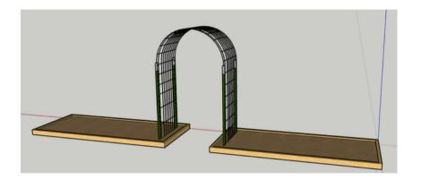
Bring the back side of the panel forward until it is in front of the T-posts. Bring the edge down until it is touching the base of the T-posts. Secure the panel to the T-posts with zip ties.
