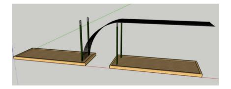
Begin to bring the panel down towards the T-posts on the other side, until the edge of the panel is touching the base of the T-post.
