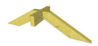
Then attach the center support to the base you completed in step 3. Screw the legs of the center seat support to the top of the 3' 6" piece, making sure to center the seat support as illustrated below (there should be about 4 9/16" on each side).
